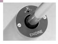
Turn adjustment pin 1 ½ turns open to provide minimum damping force. Turn adjustment pin fully closed to provide maximum damping force.
