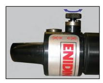
Position 0 provides minimum damping force. Position 8 provides maximum damping force. 180° adjustment with setscrew locking.
