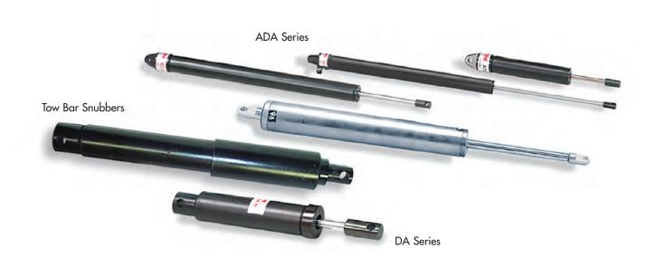
ITT Enidine Rate Controls are designed to regulate the speed and time required for a mechanism to move from one position to another. Adjustable and non-adjustable models are available to accommodate a wide variety of motion control applications. Both single and double acting hydraulic damper designs allow smooth, controllable machine operation by providing rate control for both linear and rotational (hinged) loads. Each product family offers a variety of stroke lengths from which to choose.
